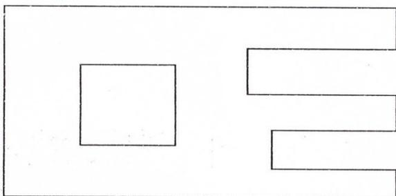
12. Copy the given sketch to 1:1 scale and dimension adopting unidirectional system with parallel dimensioning method.
