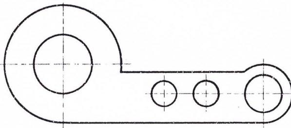
11. Copy the given sketch to 1:1 scale and dimension adopting unidirectional system with combined dimensioning method.
